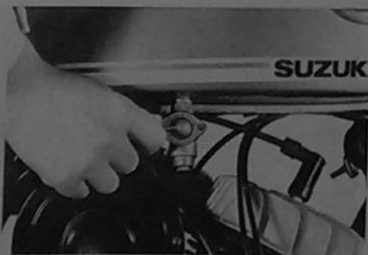
Fig. 7-2-1 Directing fuel cock lever to "0" position
