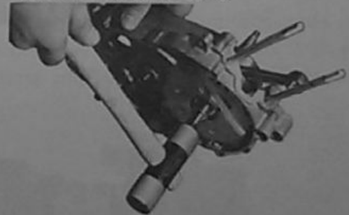
Fig. 7-3-46 Separating crankcase with crankcase separating tool (special tool No. 09910-80112)
