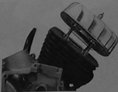
Fig. 7-3-3 Taking off cylinder head and cylinder head gasket
