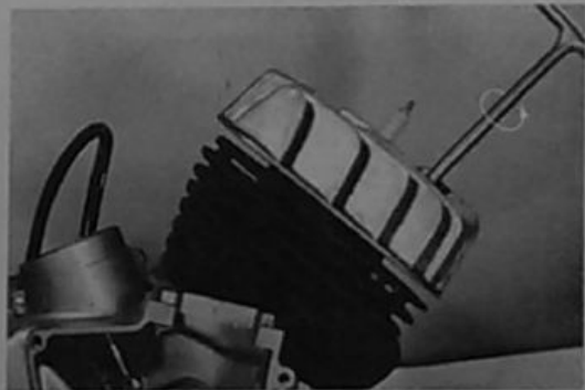
Fig. 7-3-2 Unscrewing cylinder head nuts with 14mm wrench
