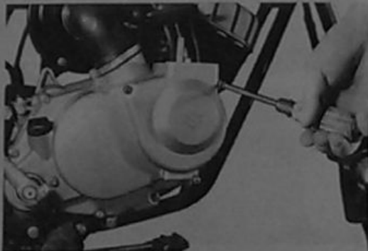
Fig. 7-2-9 Unscrewing carburetor cover screws
