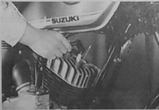
Fig. 7-2-3 Removing spark plug cap from spark plug
