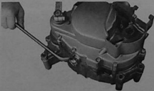
Fig. 7-3-1 Loosening drain plug with 21mm wrench
