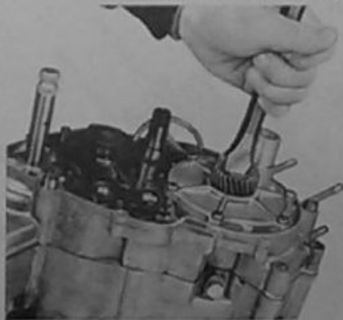
Fig. 7-3-31 Straightening primary pinion washer with chisel and hammer
