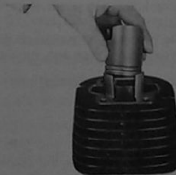
Fig. 7-5-34 Inserting piston ring into cylinder
