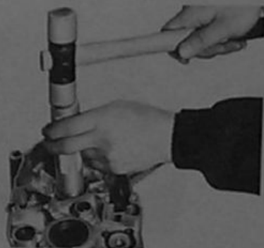
Fig. 7-3-51 Removing bearing from crankcase
