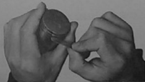
Fig. 7-5-36 Checking side clearance
