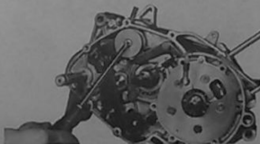
Fig. 7-3-40 Loosening gear shifting cam pin retainer fitting screw
