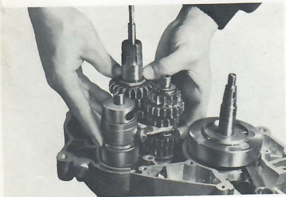
Fig. 7-4-6 Assembling transmission gear
