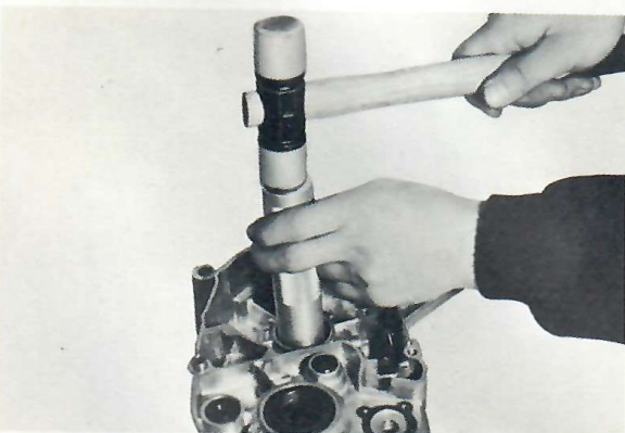
Fig. 7-3-51 Removing bearing from crankcase
