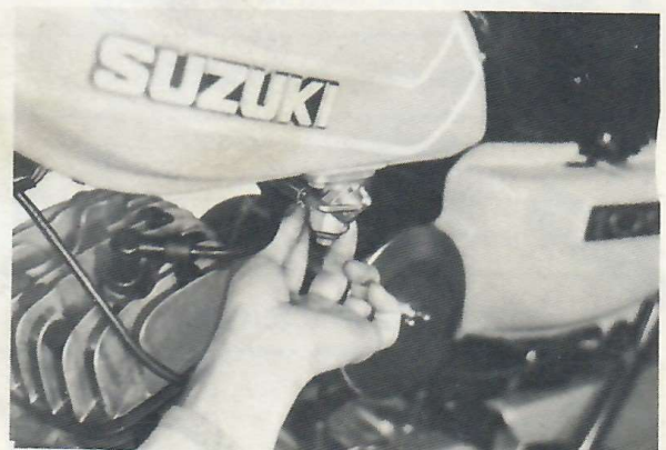
Fig. 7-2-2 Pulling fuel line from fuel cock
