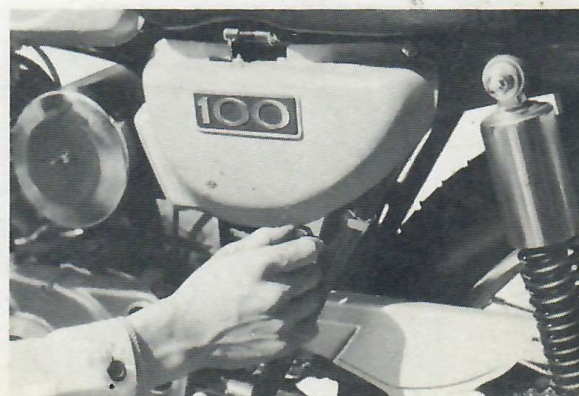
Fig. 7-2-18 Taking off frame left cover
