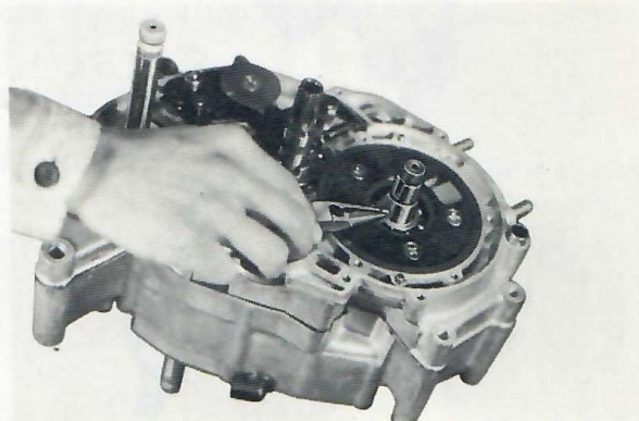
Fig. 7-3-38 Removing valve guide positioning piece from crankshaft
