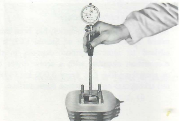
Fig. 7-5-28 Measuring cylinder bore
