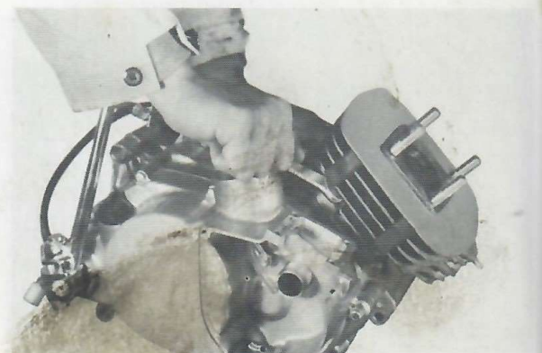
Fig. 7-3-4 Taking off cylinder
