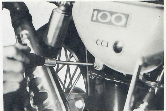
Fig. 7-2-4 Removing oil tank cover
