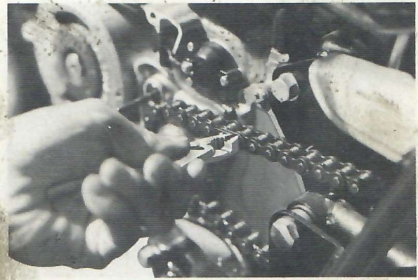
Fig. 7-2-22 Disconnecting drive chain
