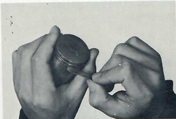
Fig. 7-5-35 Checking side clearance
