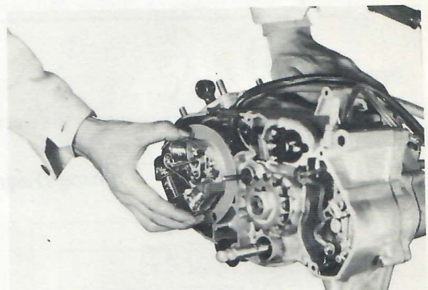
Fig. 8-4 Removing magneto stator
