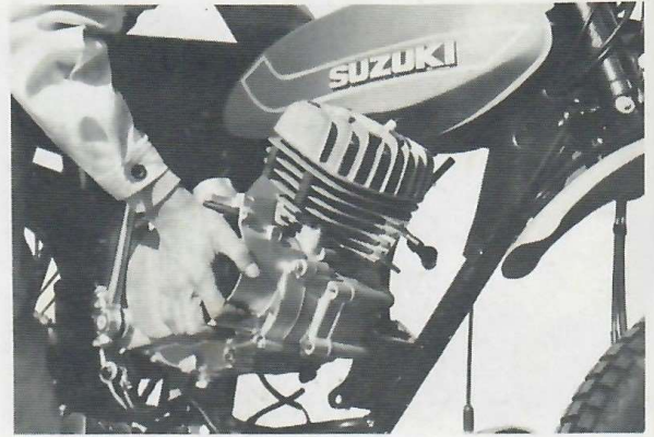
Fig. 7-2-28 Removing engine from frame
