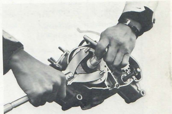
Fig. 8-2 Removing flywheel rotor
