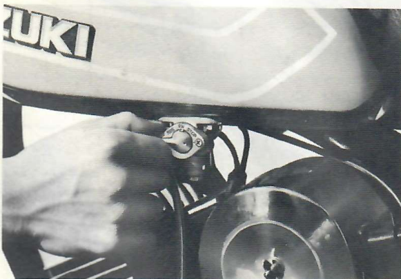
Fig. 7-2-1 Directing fuel cock lever to "STOP" position
