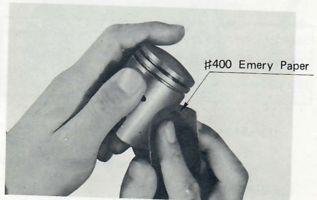
Fig. 7-5-32 Polishing piston surface
