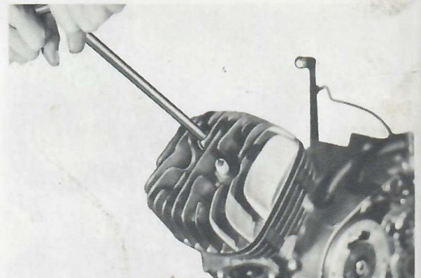
Fig. 7-3-2 Unscrewing cylinder head nut with 14 mm wrench
