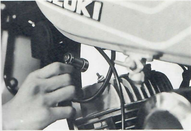
Fig. 7-2-3 Removing spark plug cap from spark plug
