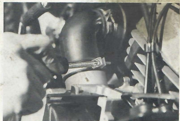
Fig. 7-2-26 Unscrewing air cleaner tube lower clamp
