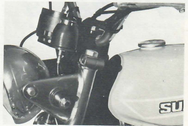
Fig. 9-1-2 Fitting inner tube to the steering stem
