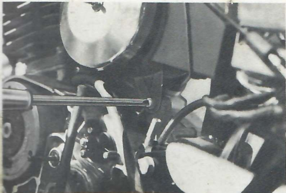
Fig. 7-2-25 Unscrewing air cleaner fitting screws
