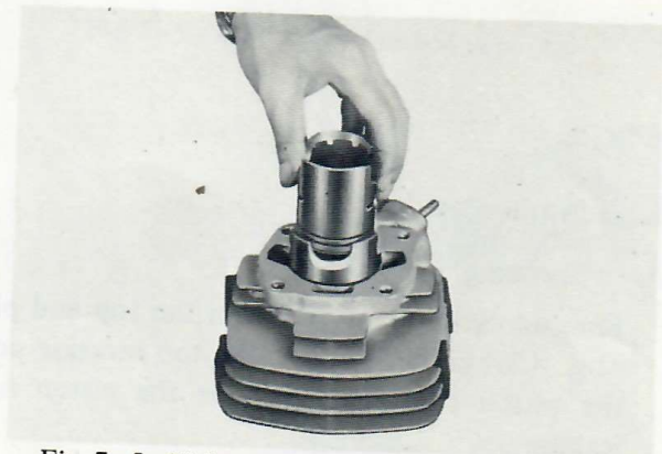
Fig. 7-5-33 Inserting piston ring into cylinder
