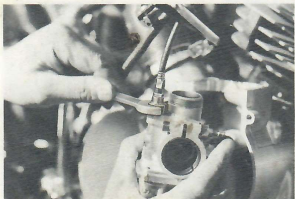
Fig. 7-2-13 Unscrewing mixing chamber cap
