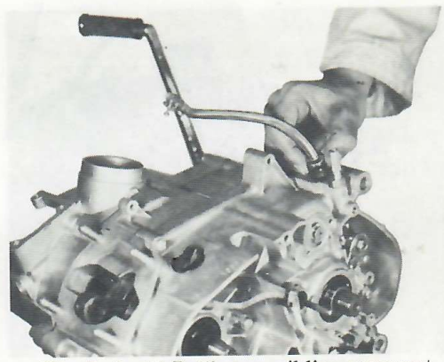
Fig. 7-3-16 Pulling up oil line grommet
